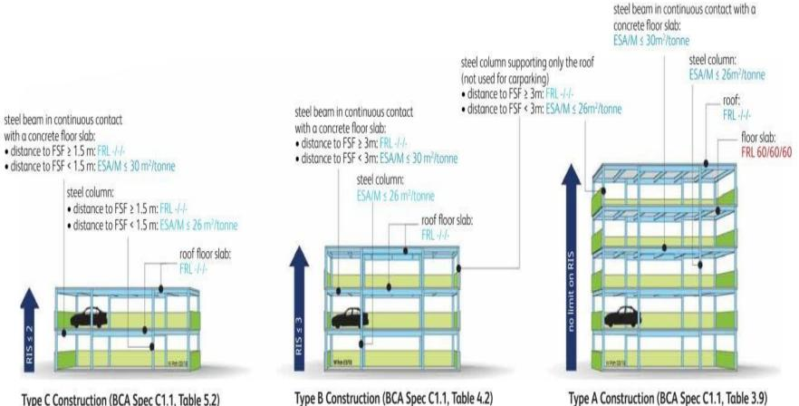
Type C Construction (BCA Spec C1.1, Table 5.2)
